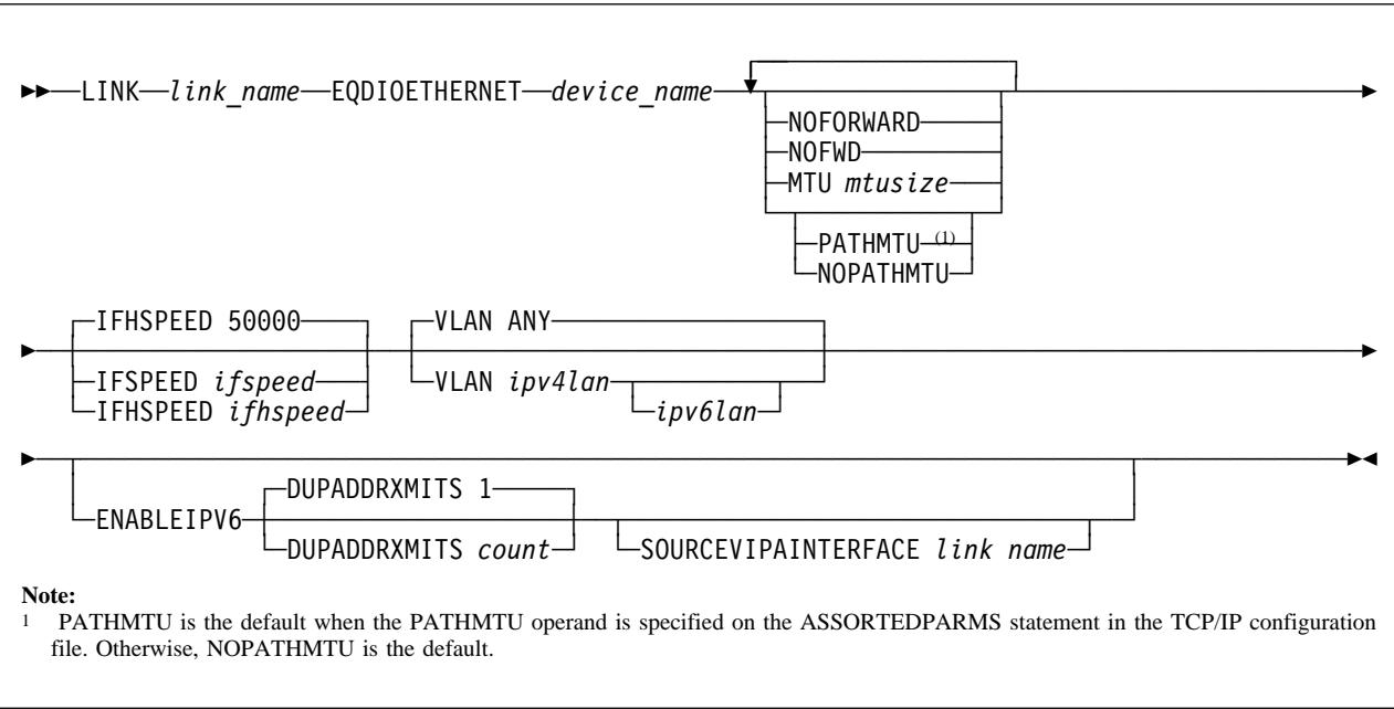
The only operands that change are that the default for IFSPEED changes to IFHSPEED 50000, and then IP/ETHERNET is removed.
