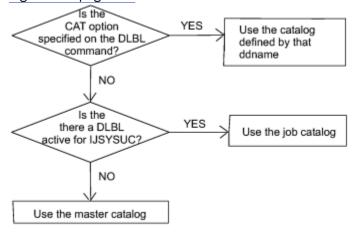
Figure 6. Determining Which VSAM Catalog to Use
