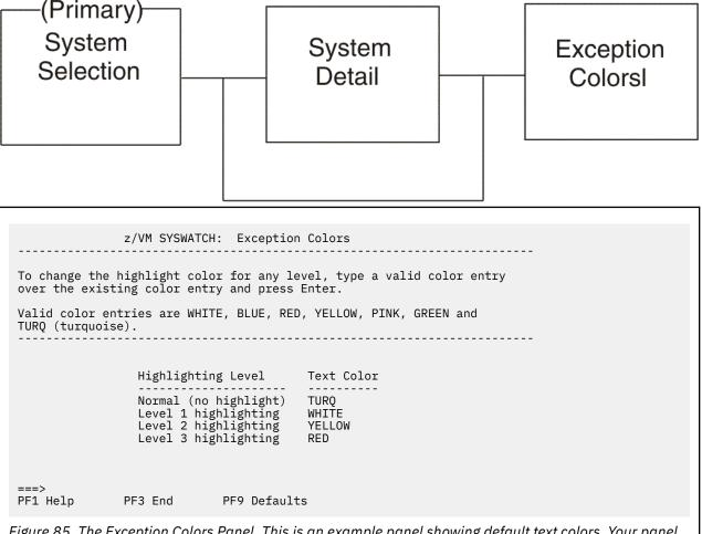
Figure 85. The Exception Colors Panel. This is an example panel showing default text colors. Your panel should look similar when displaying the default colors.
