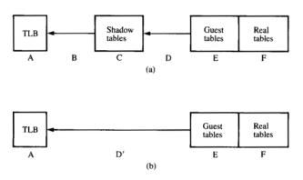
Figure 6 Translation-mechanism differences: (a) System/370 (shadow-table maintenance); (b) 370-XA (SIE).
