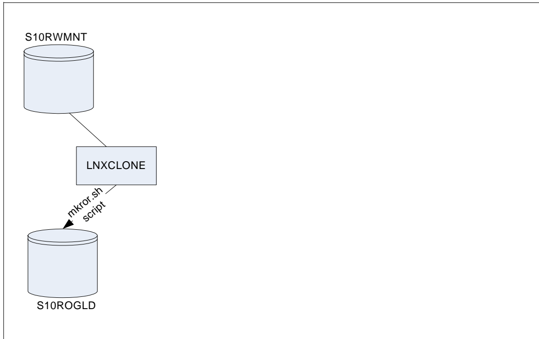
Figure 1-6 Creating a read-only root system with the mnt2rogld.sh script
