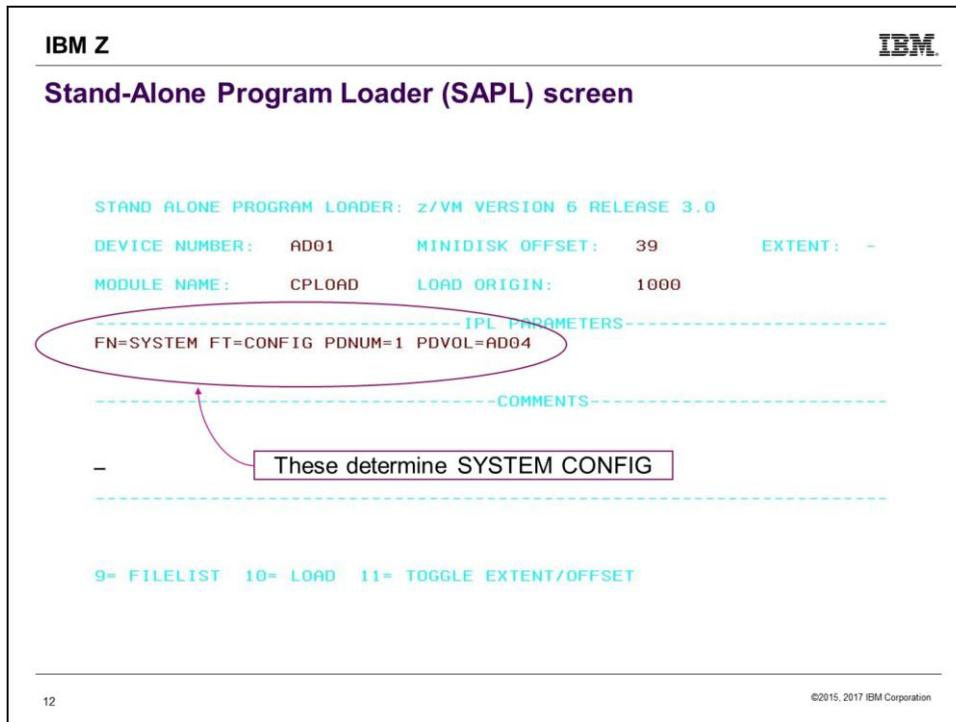
PDNUM is “PARM disk number”. PDVOL is “PARM disk volume”. So we are pointing to the PDNUMth PARM disk on DASD pack PDVOL (in this case, the 1<sup>st</sup> on AD04), and then specifying filename/filetype of SYSTEM CONFIG. Notice that the PDVOL is *\*not\** the same as the load address in this case.
