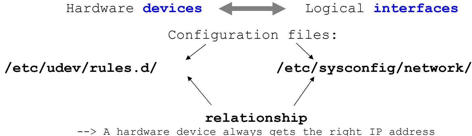
Devices are configured via udev (framework for dynamic device configuration)
