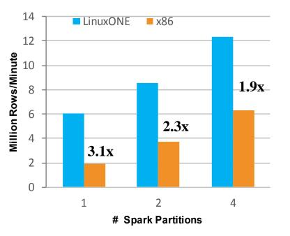
Test ran one LinuxONE guest, RHEL 6.5 on LinuxONE & z/VM 6.3 with 32 vCPUs (16 cores with SMT) and 512GB memory, Spark 1.5.0, IBM JDK1.7-SR3
