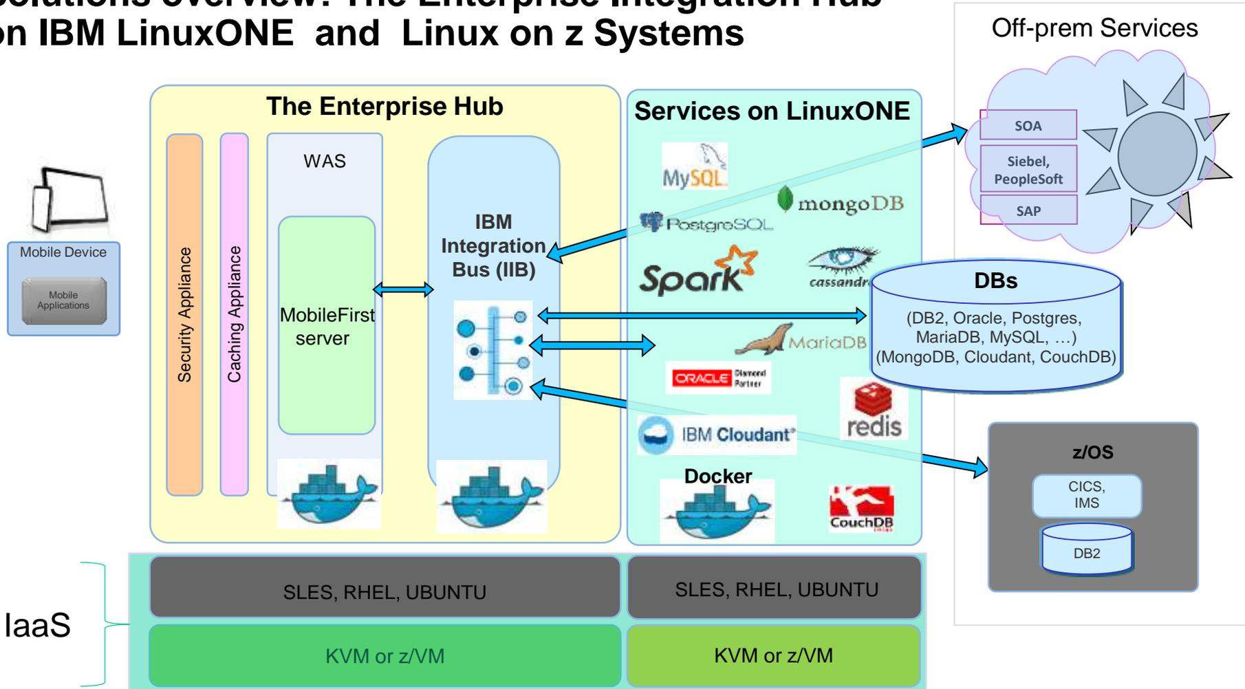
**IBM Integration Bus** can help you simplify the connectivity between your IT assets, including legacy apps, packaged apps and web services, without requiring coding changes. It provides content and context based routing that helps you manage and simplify business-critical processes. It enables you to integrate Open Source technologies and Hybrid cloud with most of your existing IT assets quickly, simply and at a low cost.
