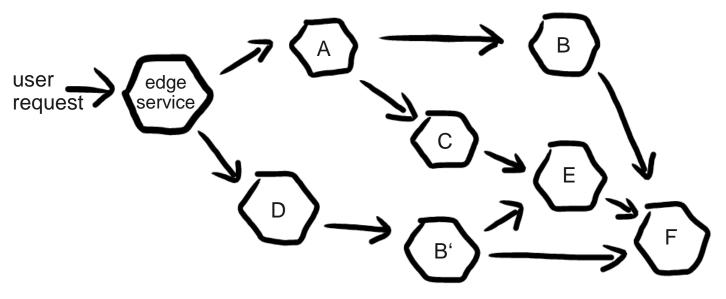
Network latencies add up in meshes of microservices z Systems: large complex with in-box networks reduces latencies
