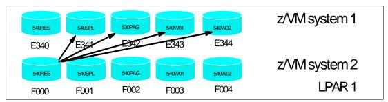
Figure 4-13 The problem with two z/VM systems with identical volume labels
