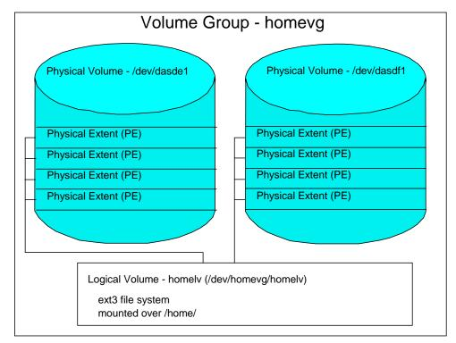
Figure 11-1 LVM block diagram
