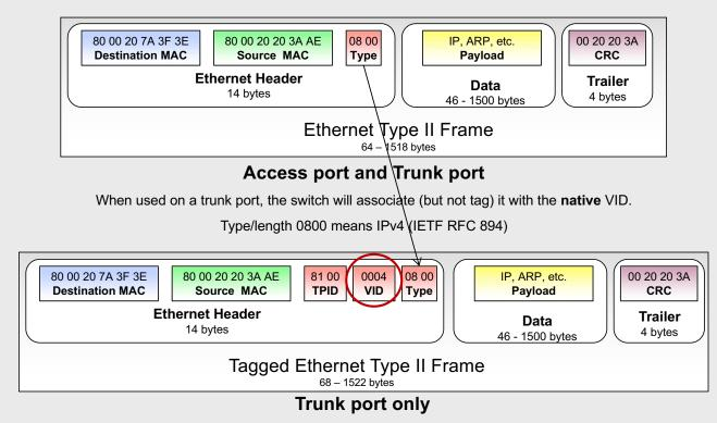
Value 8100 in the Type field means a VLAN tag follows, followed by the actual type/length field
