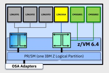
The Port-Based Vswitch allows a guest with multiple vNICs to connect via ACCESS ports to a single VLAN-aware virtual switch
