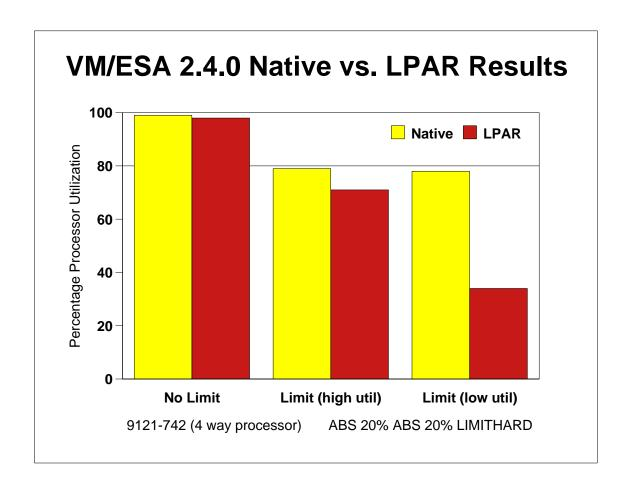
Note however, that in LPAR environments, the scheduler limit settings can not be as accurate. Shown here is the same VM/ESA 2.4.0 system running native and in an LPAR. For the LPAR tests, two partitions were defined both as logical 4 ways. The system under test had a weight of 30 with the other system having a weight of 70. As you can see the limited user received less than what they did in native systems.
