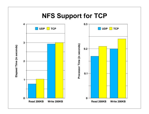
As mentioned earlier NFS added support for TCP connections. The two charts on this page show the difference with the NFS for VM/ESA 2.4.0 between UDP and TCP. The chart on the left shows elapsed time. For the read scenario, TCP does add to the elapsed time by about 34%. However, since write processing elapsed time is dictated greatly by the NFS protocol, the use of TCP does not increase the elapsed time for writing files as greatly.
