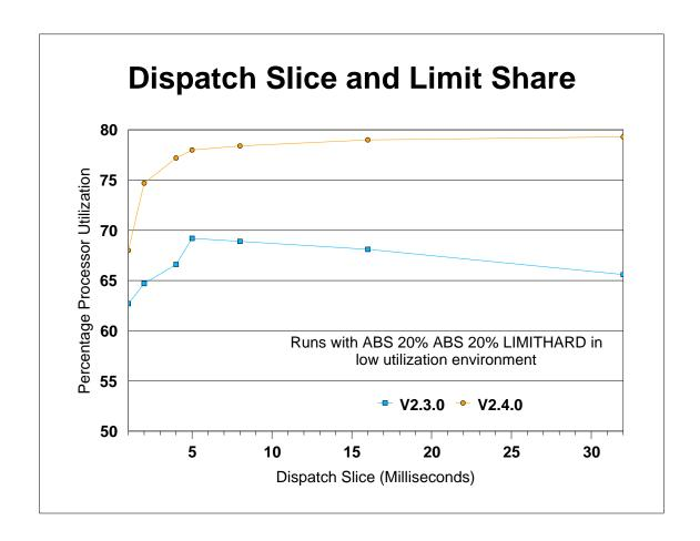
Experiments were also made with the LIMITHARD setting with various minor dispatch slice times. In VM/ESA 2.3.0, very short or very long minor dispatch slices made the limit tracking less accurate. This has been improved somewhat in VM/ESA 2.4.0.
