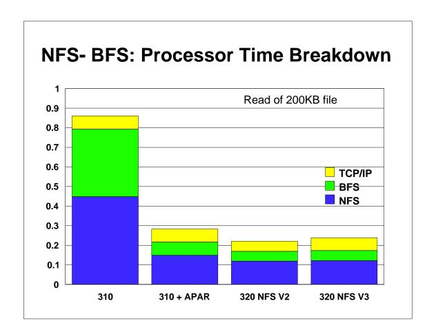
This chart shows the breakdown in processor time to read a 200 KB file from the BFS on VM through NFS. You can see that the TCP/IP portion stays about the same. The bulk of the improvements were in the interface between the NFS machine and the BFS server. The use of NFS version 3 protocol does not improve things in this particular scenario.
