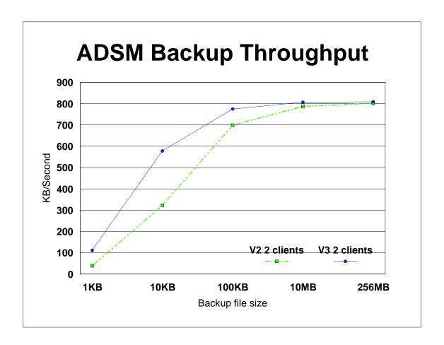
This chart shows backup throughput also, but with 2 clients being used. Remember that in all cases version 3 clients were used. Again you see that ADSM version 3 is the better performer. Limitations on our network and processor speed help lead to the leveling off of performance.
