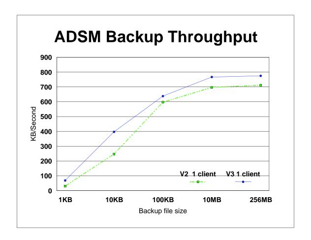
This graph illustrates that the largest improvements in backup throughput were for smaller files. However, the greatest aggregate throughput is for large files. The measurements were made with only original backups, and not subsequent backups. In all the measurements shown here, only a single client was involved.
