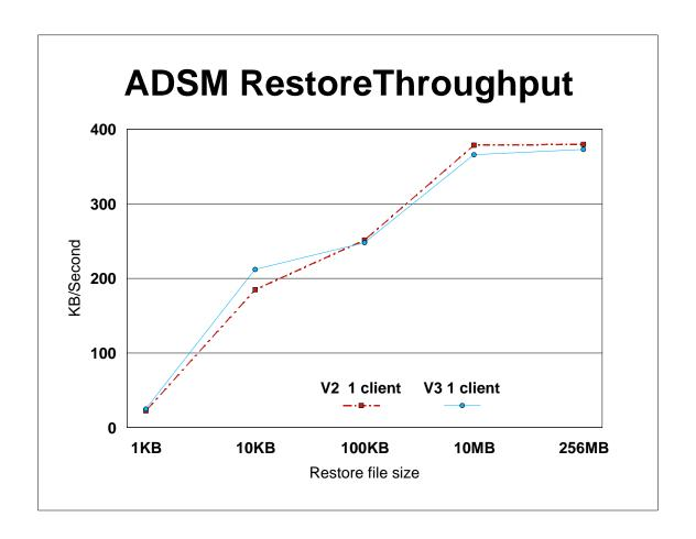
ADSM Restore throughput did not change significantly in version 3 for any file size. These measurements were made with a single client. If you compare back to the throughput graphs for backup, you will note that restore throughput is much lower.
