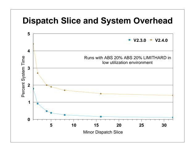
Another interesting point from these tests with varying minor dispatch slice times was the system overhead. In general, the improved accuracy of LIMITHARD settings costs more in system time. Thought in non-limited cases it stays the same.
