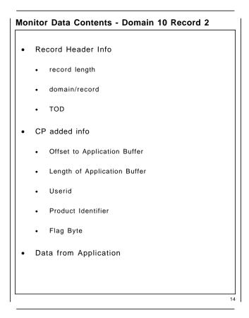
There are three parts to Sample Record for APPLDATA. The first is just the normal record header info. Note the TOD, we'll use that later.
