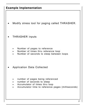
Talk is cheap, so lets try a real example. We (performance evaluation) have a program to help stress the paging system. I've modified it to use APPLDATA. It will collect 4 items. The first two are just initialization or config data. The second two are the two items we talked about earlier: Accumulator of times thru loop (Running count of requests) and Accumulator of time to reference pages (timing of requests). Later we'll throw in TOD to get the other things I talked about.
