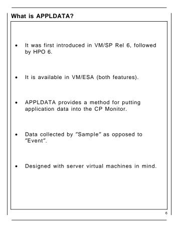
APPLDATA was introduced in VM/SP 6 for support of SFS and is also used in HPO 6. With VM/ESA, it is available in both features. There are some differences which will be pointed out.
