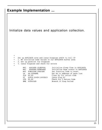
This sample of code shows the setup and issuing of the Diag DC. First we initialize the constants in the buffer, set the function code to start, and then issue the Diagnose. My example program does do nominal error checking for Diag DC.
