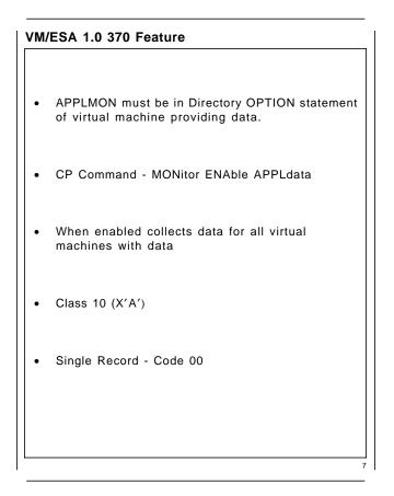
This foil gives the basics of APPLDATA in 370 feature (also SP and HPO 6). To be allowed to produce APPLDATA, a virtual machine must have the APPLMON operand in the directory OPTION statement. The CP Monitor command was extended to include the new class of APPLDATA. In this class there is a single record.
