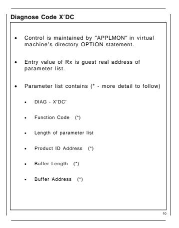
The APPLMON entry in directory OPTION statement is what allows you to issue Diagnose x'DC'. Diag DC is structured like most diagnoses, with the Rx register pointing to parameter list with above items.
