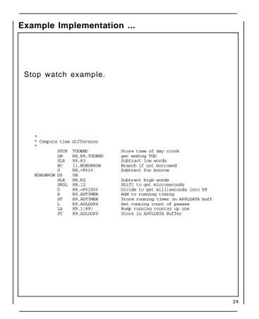
Registers 2 and 3 contain the TOD from when we started the request. In this code section, we first get the ending TOD via STCK into Register pair 8 and 9. This code shows how to subtract the two. It then goes on to get the delta into more manageable units (microseconds to start, and then milliseconds). Value is stored into APPLDATA buffer (ADTIMER) along with the loop counter (ADLOOPS).
