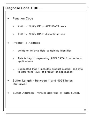
The function code is the flag for CP of whether you (the application) are interested in data collection. The wording in some manuals is a little confusing. It says Start is "Start Interval Recording", this doesn't mean CP will at that very moment cut a sample record. It only means CP will include this APPLDATA at the next sample interval. More on this later.
