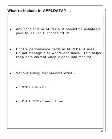
Some APPLDATA specific thoughts. Constants should be set in APPLDATA buffer before Diag DC since CP could sneak in between Diag and initialization. Update the values right in the buffer. If you keep them else where and move them, there can be anomalies caused by timing between CP sampling and your moving of the data.
