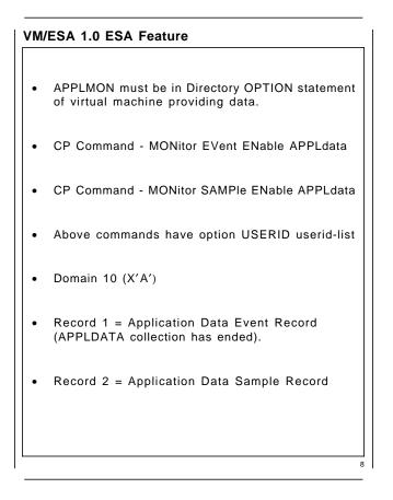
In the ESA feature, again APPLMON must appear in the OPTION statement. Both the Monitor Event and Sample commands were extended to include the new domain (ESA monitor uses domains, not classes). There are two records in this domain.
