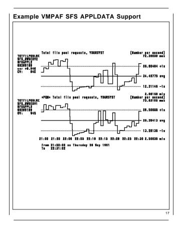
This is an example of VMPAF support for SFS APPLDATA. In addition to all the counters and timings put in APPLDATA that VMPAF exposes, there are several pre-defined equations that make analysis easier. This example shows the file pool request rates for each of the two file pool servers. VMPAF could be used to compare any of the APPLDATA statistics with any other monitor (or other source) available.
