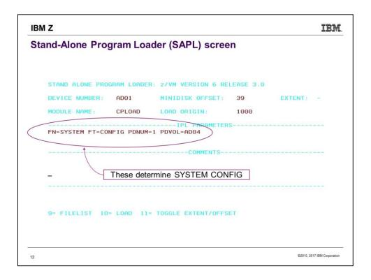
PDNUM is "PARM disk number". PDVOL is "PARM disk volume". So we are pointing to the PDNUMth PARM disk on DASD pack PDVOL (in this case, the 1<sup>st</sup> on AD04), and then specifing filename/filetype of SYSTEM CONFIG. Notice that the PDVOL is \*not\* the same as the load address in this case.
