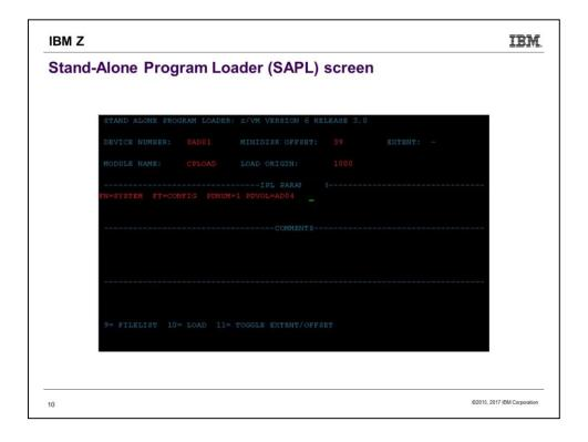
When your LOAD completes (may take only a few seconds, could be minutes) you see the screen of the Stand Alone Program Loader. The SALIPL utility was used by Install to fill in the details.
