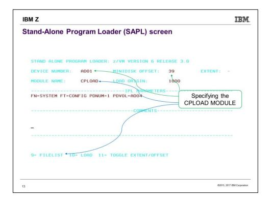
Use the file CPLOAD MODULE on the minidisk that starts at cylinder 39 on DASD AD01. The device number was filled in for you by virtue of choosing it on the HMC Load Screen. As an alternative to accepting CPLOAD or knowing the name of another CP version, you can mash PF09 to see a FILELIST of all the files on the indicated minidisk, and choose from among the MODULEs you see there.
