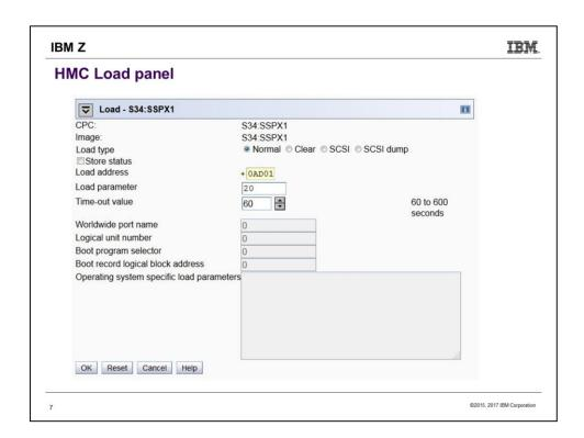
This is typical appearance of the load panel on the Hardware Management Console (HMC). The parameter values originally came from customizing the Activation Profile of the LPAR, but they're saved from whatever was used most recently.
