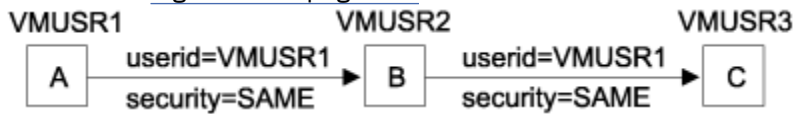
Figure 92. Access Security User ID of User Program Flowed from VMUSR1 to VMUSR3
