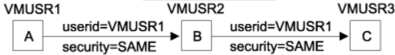
Figure 93. Access Security User ID of User Program Flowed from VMUSR1 to VMUSR3
